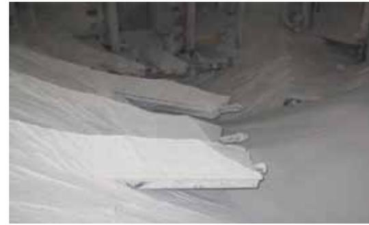
Inside the 'bomb shelter', all slides lead into here and feed the alumina onto a conveyor.
