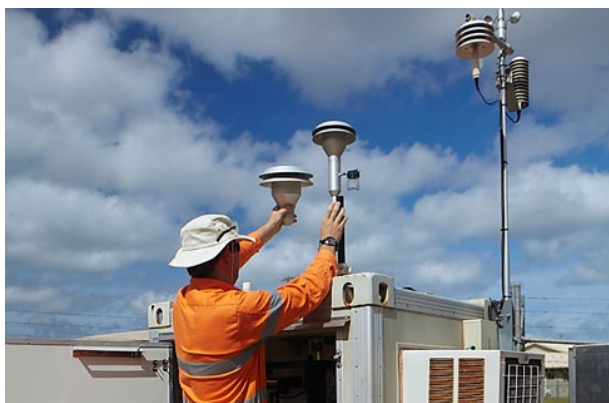
Figure 45. Rio Tinto Weipa Dust Monitors
