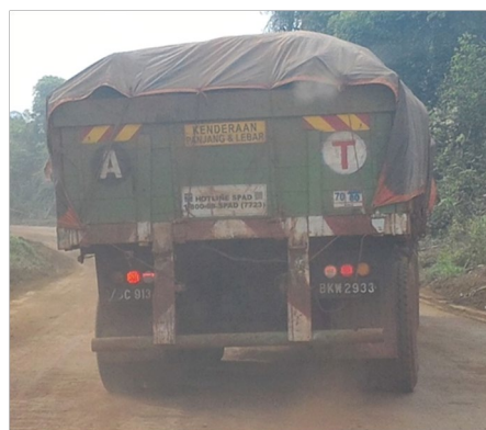
Figure 28. Poorly Loaded Truck with Non-Secure Cover
