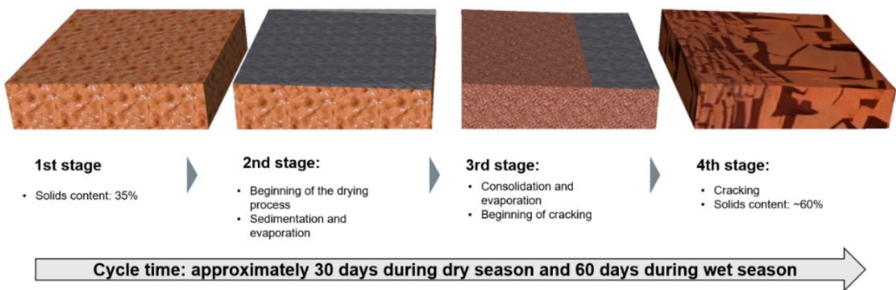
Figure 55: Tailings desiccation process
