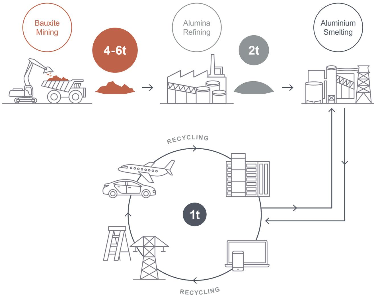
Bauxite is the primary ore from which aluminium is extracted. Alumina refineries process bauxite ore to produce aluminium oxide or alumina, by dissolving the bauxite in a caustic solution at high temperature and pressure; and then precipitating the dissolved pure alumina.
