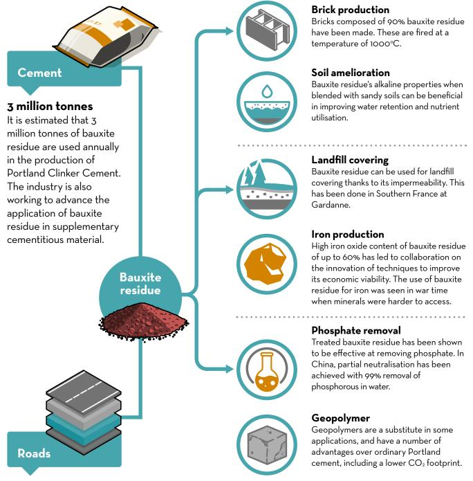
When bauxite residue is dewatered, compacted and mixed with a suitable binder, it can make a building material for haul roads.
