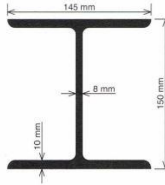
Aluminium Beam 10.6kg/m
