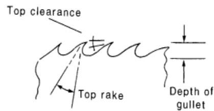
Tungsten-Carbide-Tipped Blade Circular, with coarse chip-breaker teeth
